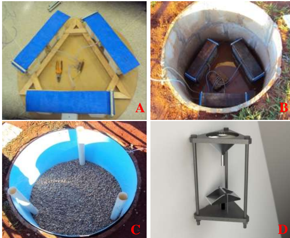
Figure 2. Details of the structure and mounting of the hydraulic lysimeter. (A): hydraulic load cells arranged in an equilateral triangle format and attached to each other by a metal connector. (B): arrangement of hydraulic load cells supported on concrete foundations in the field; (C): mounting the lysimeter in the field, with layer of gravel and the tubes to the drainage system. (D): tipping bucket rain gauge adapted for measuring the water drained.
